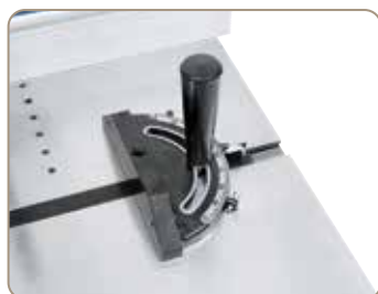
Mitre fence moveable along entire table length.
