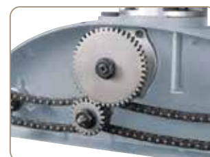
Rearrangement of gear wheels allows for easy speed change.
