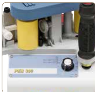
The required working temperature is set by potentiometers.
