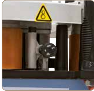
Easy adjustment of most commonly used bands (0.3 / 1 / 2 / 3 mm in width)
