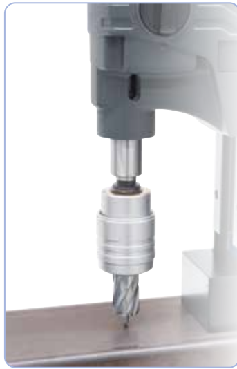
Core drilling with quick release tool holder
