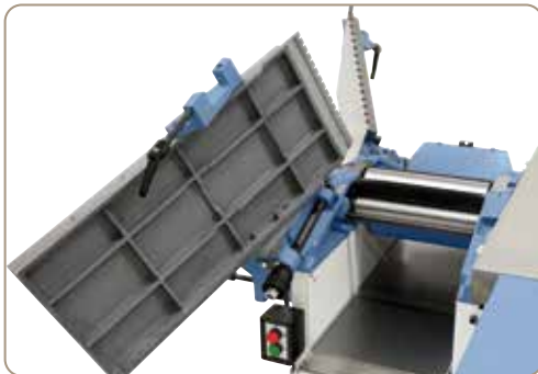
The planer tables tilt into upright position to allow for optimal and safe working conditions even when thickening short workpieces.
