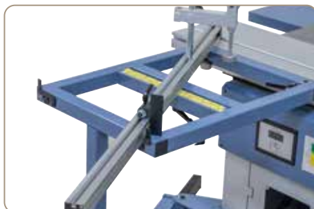
The torsion-free square table assists when cutting large panel.
