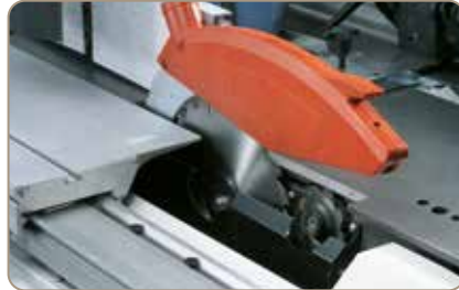
Sawblade cover with integrated dust port connected at riving knife.
