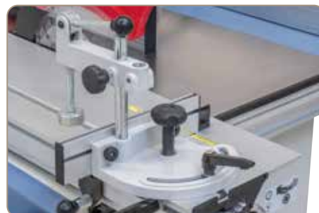
T-slot in sliding table allows mounting of mitre fence and end stop.
