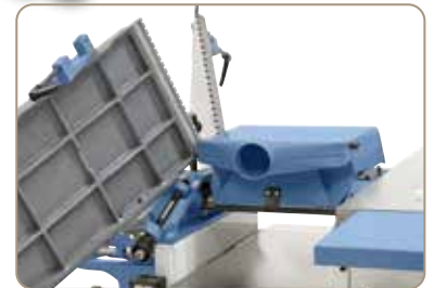
Integrated, tiltable dust hood - extraction outlet 100 mm.
