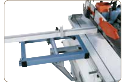
Square table can be moved along the entire length of sliding table.
