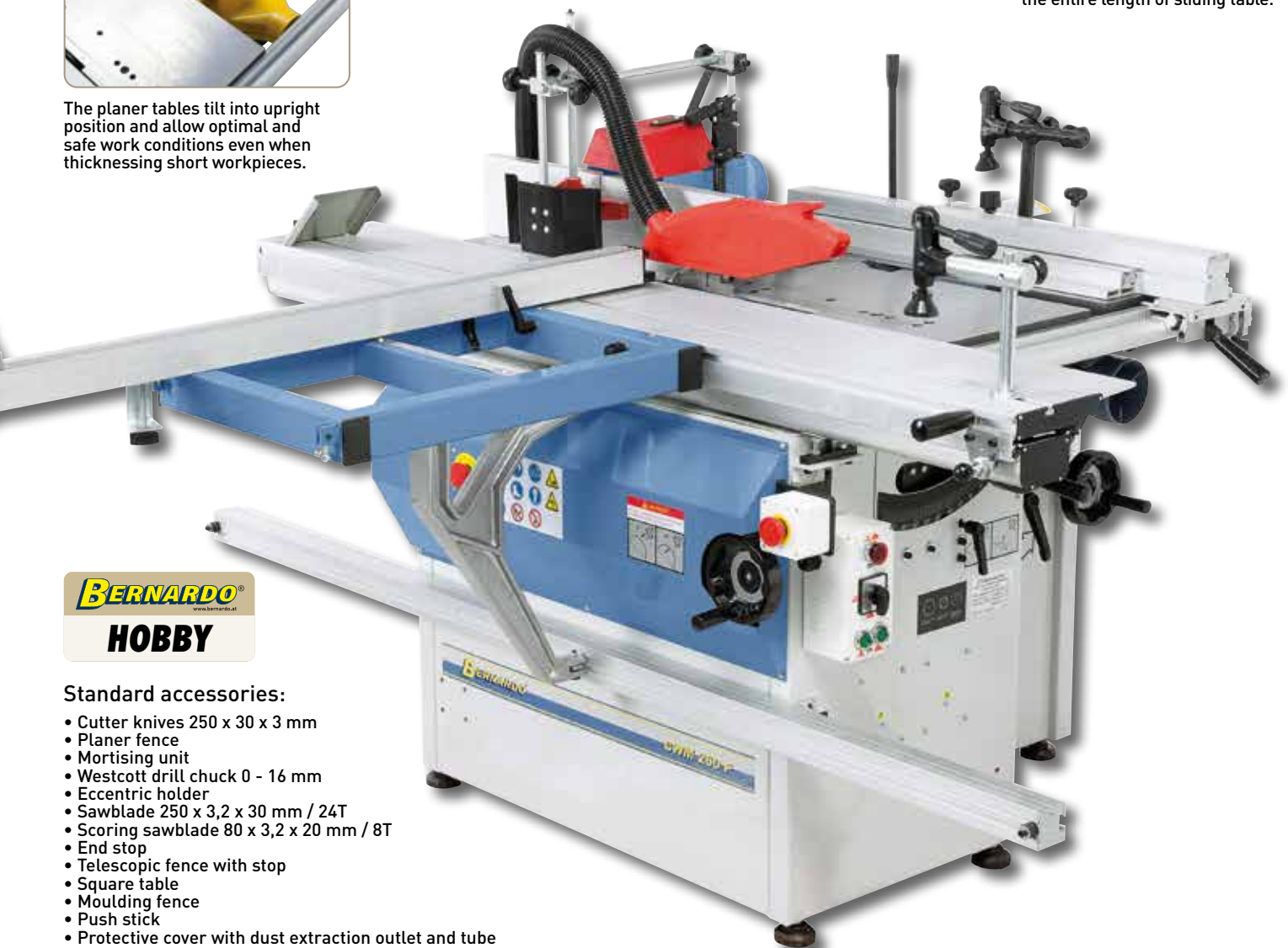
Square table can be moved along the entire length of sliding table.
