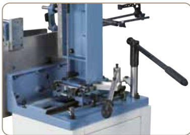
Cross and longitudinal movement feature adjustable fences.
