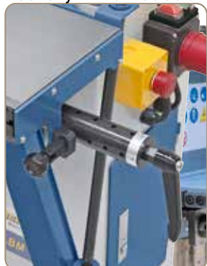
Precise roller guiding allows accurate movement of drill unit.
