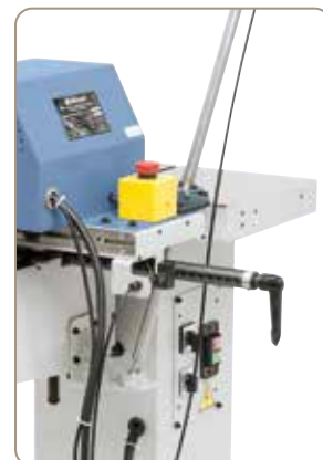
Rotor group with grid spacing 16 / 20 / 22 / 25 mm includes remote lever to set spacing, ideal for multiple hole drilling.
