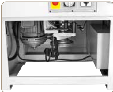
Amply sized opening on machine front allows for easy belt change to adjust speed.
