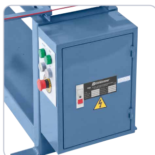
Clearly arranged switching and operating elements on the side of the machine body.
