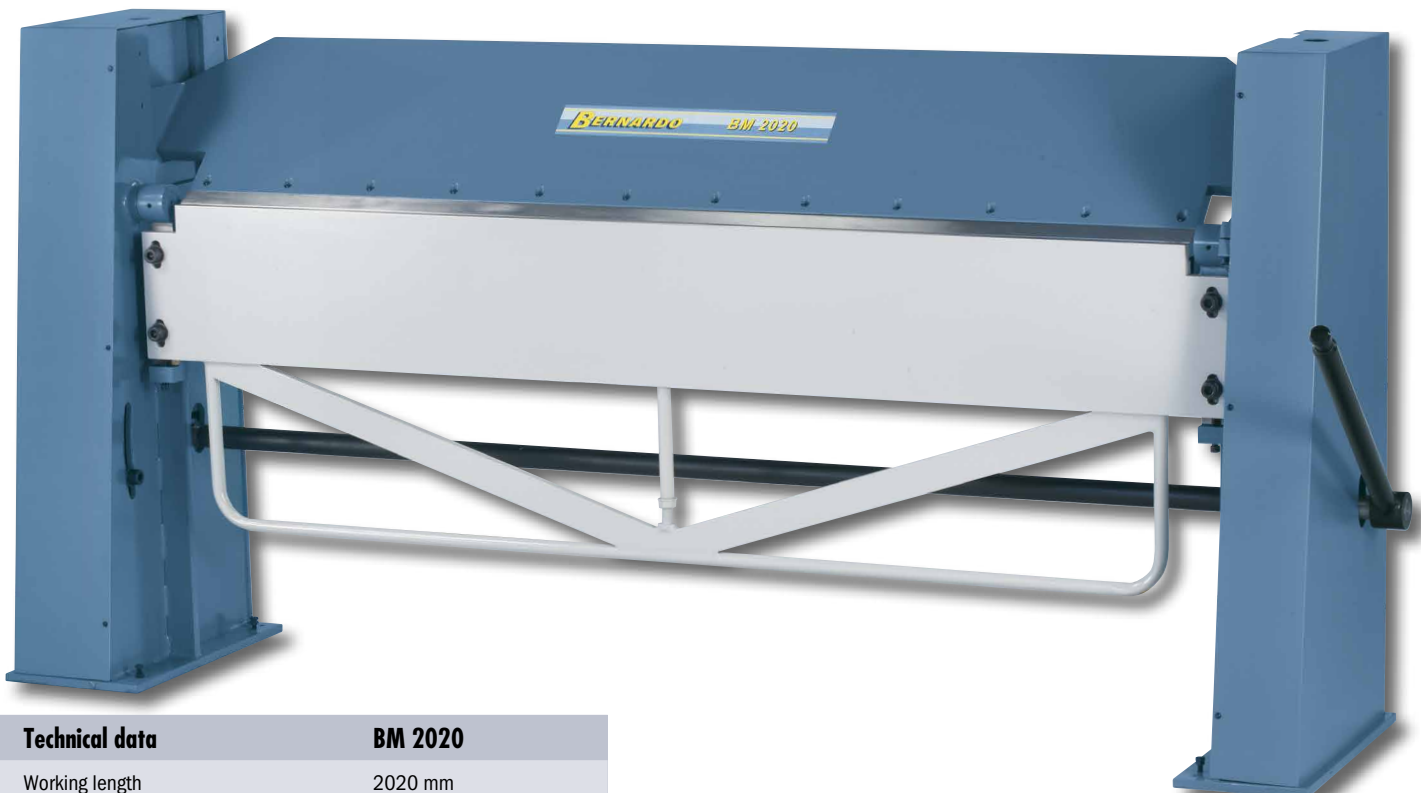
Large dimensioned guide guarantees exact bending.
