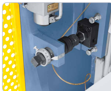
Easy adjustment of the cutting gap to the respective sheet thickness at the back of the machine.
