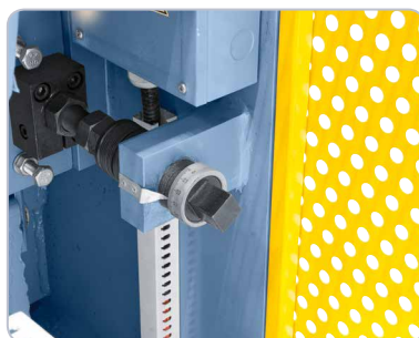
Easy adjustment of the cutting gap to the respective sheet thickness at the back of the machine.
