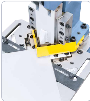
Adjustable stops with scales, ideal for serial production
