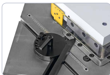
Exact adjustment of the stops by integrated scales in the machine table.
