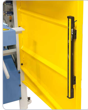
Sick-light barrier on the backside of the machine (optional)
