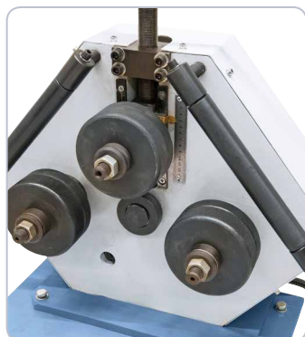
The adjustment of the upper roll is read via a mm-scale.
