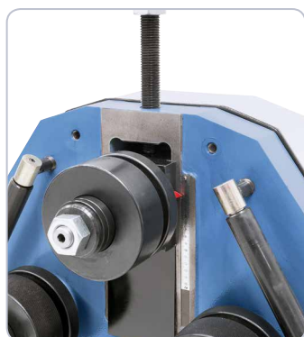
Stable guiding of the upper roll, adjustable via mm scale.
