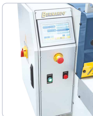
Control Fuji with touch screen comes standard.
