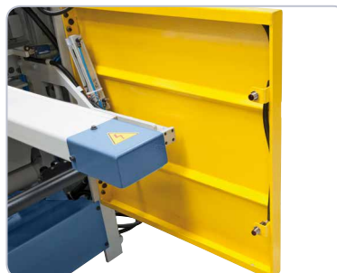
The side protective plate and photocells prevent interference in the running machine.
