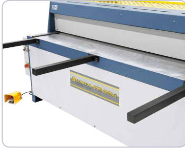
The support arms facilitate the processing of large format sheets.
