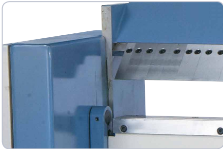
Large opening of 100 mm (with segments).
