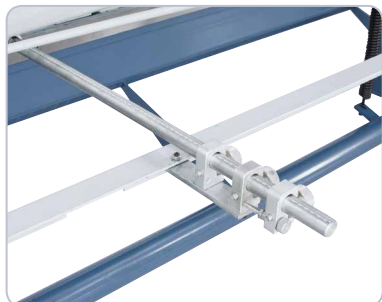
The backgauge with fine adjustment is ideal for serial production.
