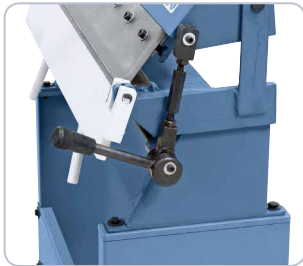
Special clamping device for secure clamping.
