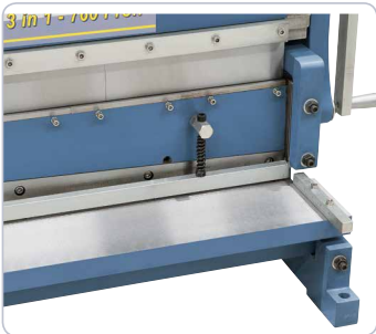
Support table with right-angled stop on both sides.
