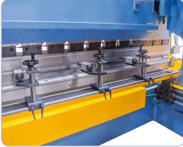
3 pcs. height-adjustable backgauge fingers, laterally adjustable via linear guide
