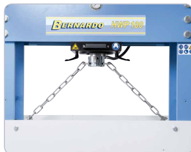
Including device for height adjustment of the work table.
