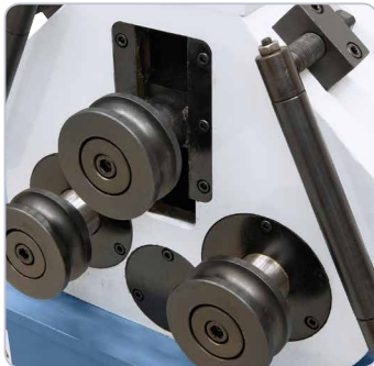
Guiding of the upper roll by precision ground guide rails.
