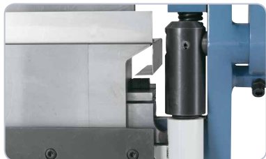
Standard with goat-foot segments, ideal for bending of e.g. boxes.
