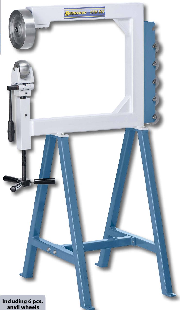
Practical holder for the anvil wheels on the side of the machine body.
