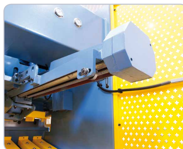
Backgauge with ball screw for increased accuracy.
