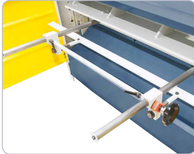
Standard with backgauge, ideal for serial production.
