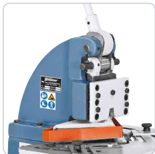
Mechanical power transmission by means of eccentric.
