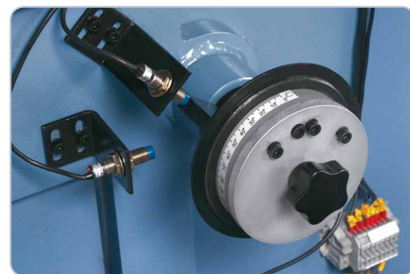
The setting of the desired bending angle is done by a scale ring.
