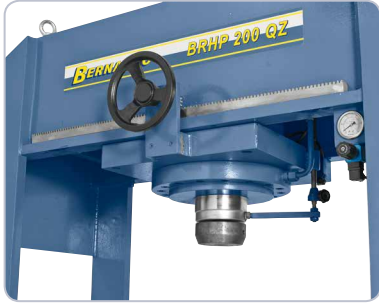
The piston can be moved to the left or right by handwheel.
