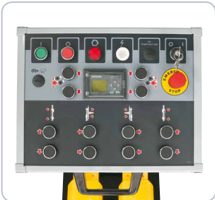
Control panel BPK 80 H with hydraulically adjustable guiding rolls (option).
