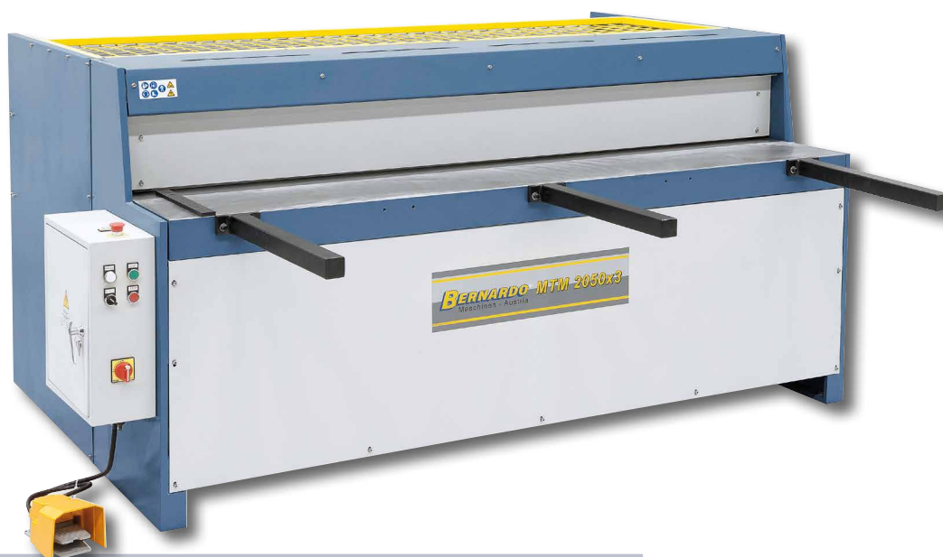
The standard light barrier prevents intervention in the running machine.
