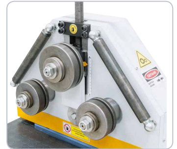
The lateral guiding rolls can be steplessly adjusted to the respective profile.
