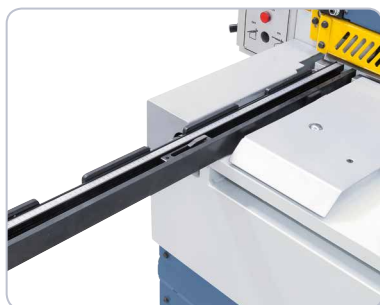
Exact work through lateral stop ruler with integrated scale.
