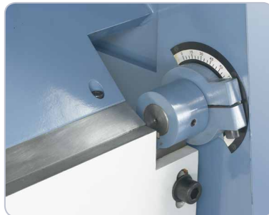
Setting of the bending angle by means of scale
