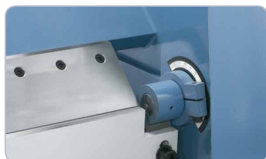
Fast and easy adjustment of the bending angle via an easy-to-read scale.
