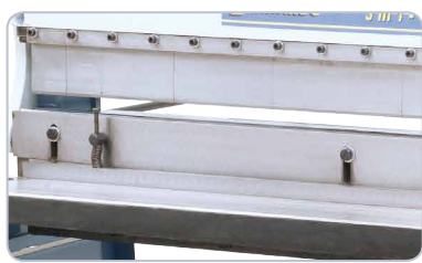
The removable inserts result in a high number of bending possibilities.
