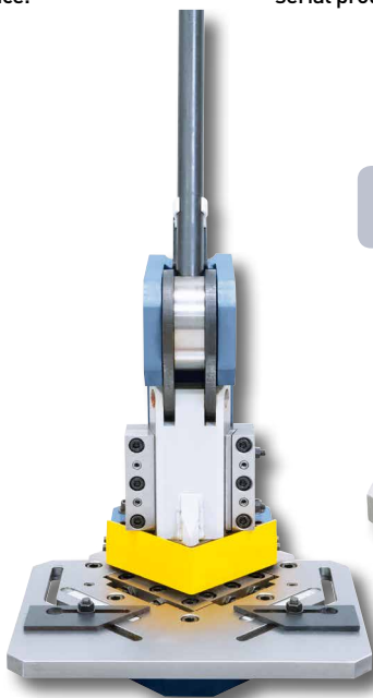
Guidings are adjustable free of clearance.
