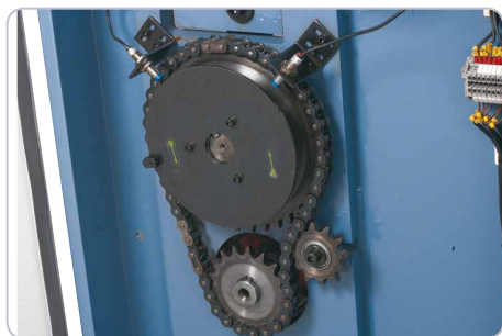
The robust chain drive ensures exact movement of the upper beam and clamping of the workpiece.
