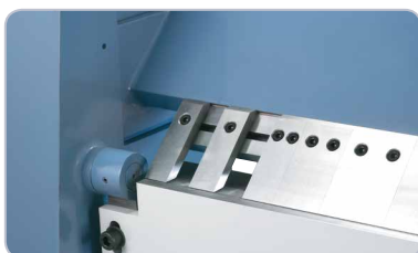
The high upper beam allows the production of high-edged profiles, hardened and ground segments.
