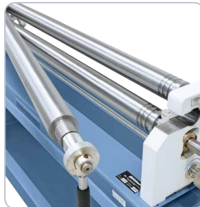
The swivelling top roller facilitates the removal of the finished workpiece.
