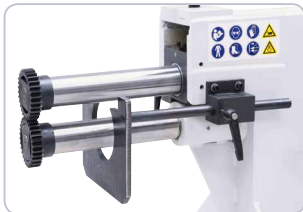
Adjustable fence for precise work and high repeatability
