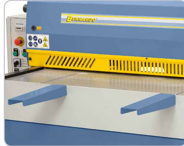
Front sheet supports for processing large format sheets.
