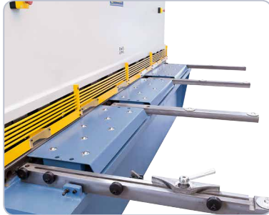
Front sheet supports with integrated rolls for processing large format sheets.
