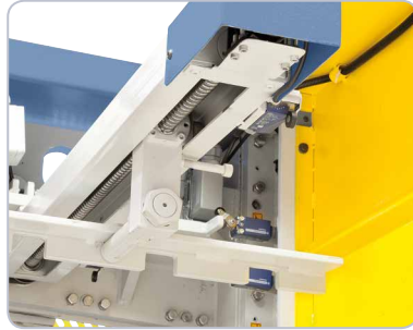
Backgauge with ball screw for increased accuracy.
