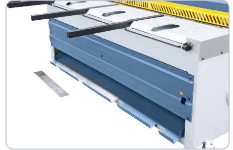
Collecting tray for the sections on the frontside of the machine.
