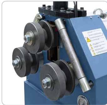
Standard roll set suitable for bending a wide variety of profiles.
