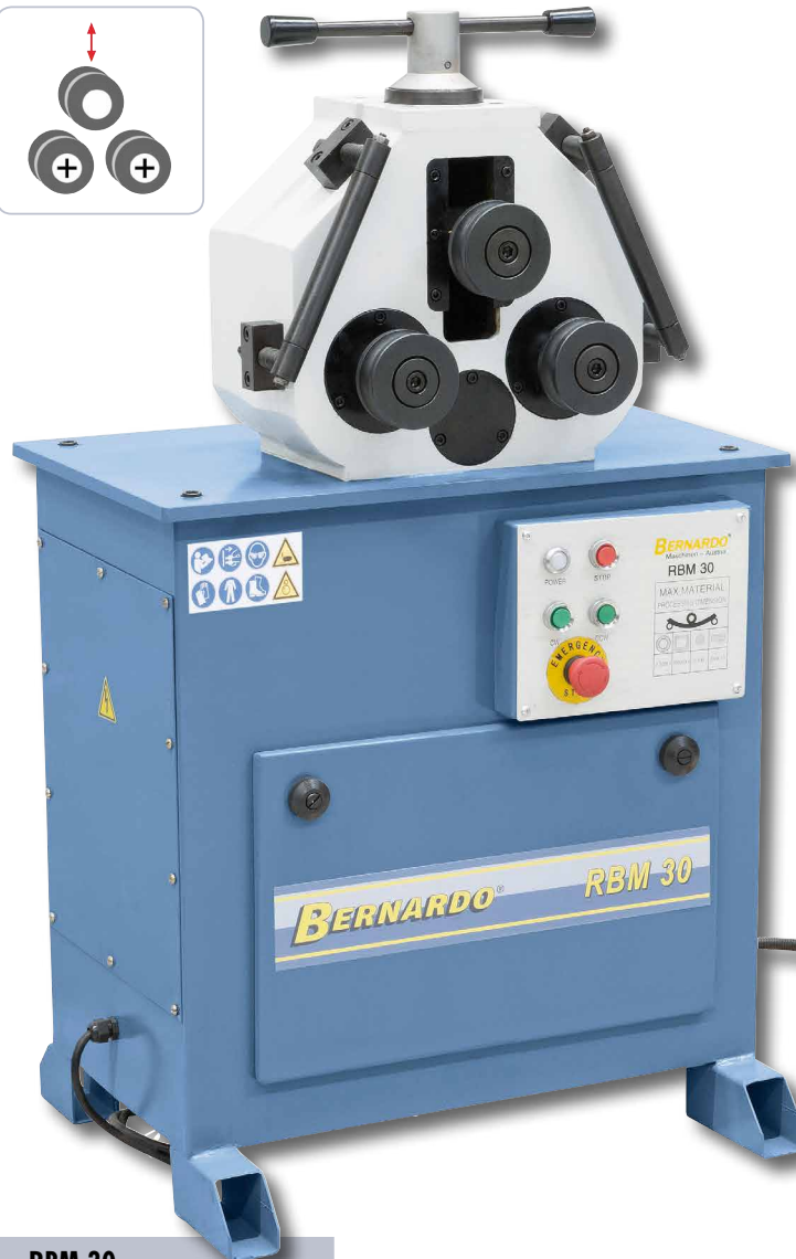
Guiding of the upper roll by precision ground guide rails.
