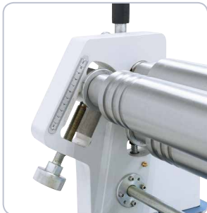
Exact adjustment of the back roller by scale.
