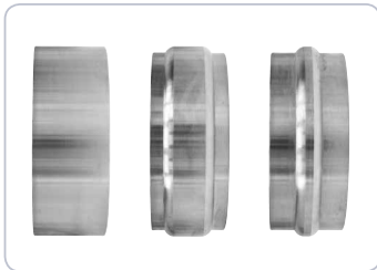
Serially: 1 pc. roller wheel for wheeling 2 pcs. roller wheel for making beads
