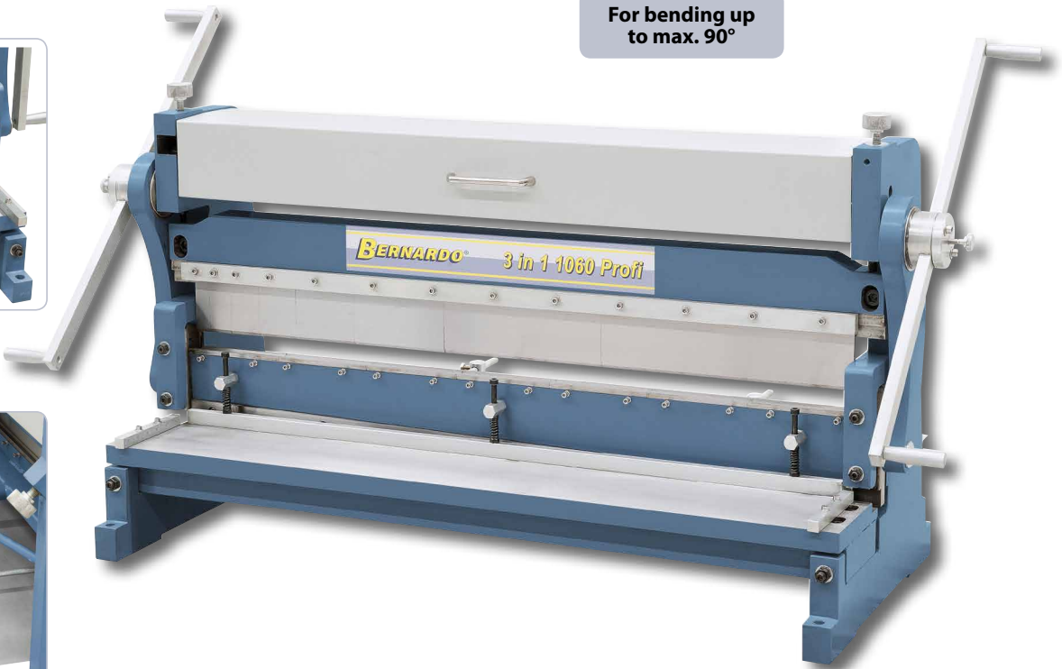
Support table with right-angled stop on both sides.
