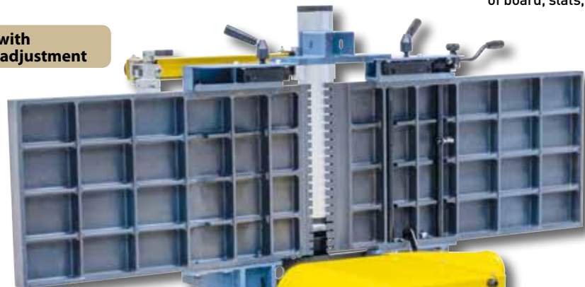
Simultaneous folding of planing tables ensure maximum comfort.
