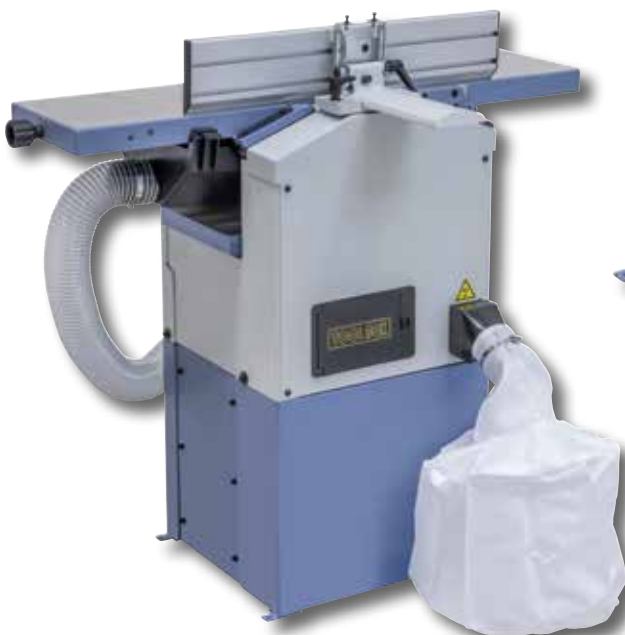
Serially equipped with integrated dust extractor and filter bag.
