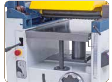
Solid thickening table with spindle guide and support for accurate planing of board, slats, planks etc.
