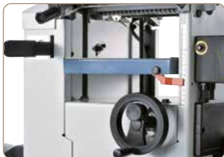
Thickening table is guided on four threads. The height can be read on the scale.
