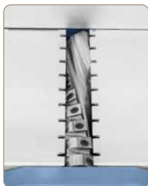
The table is designed with slots on both sides and a spiral cutter head to minimize the noise level.
