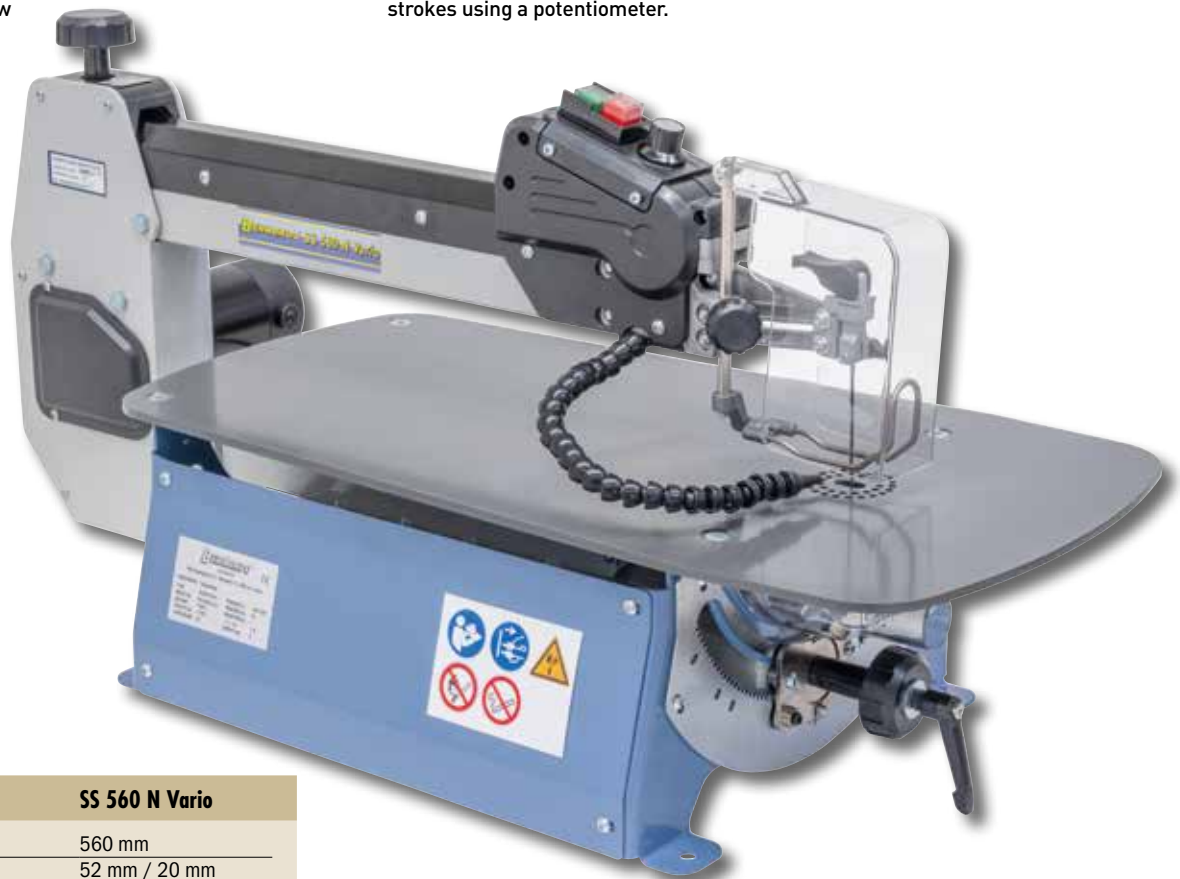
Tilttable saw bow from -30^{\circ} to +45^{\circ}
