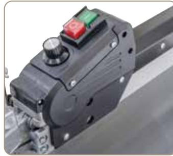
Stepless adjustable number of strokes using a potentiometer.
