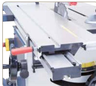
The sliding table features a generous size and runs smoothly on hardened prism guide ways.
