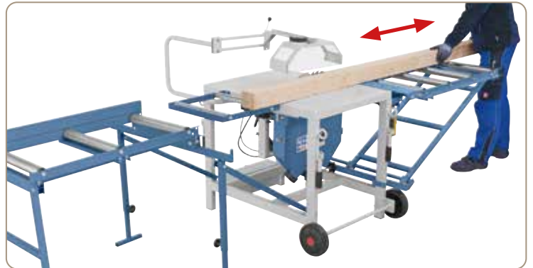
Parallel separation cut
