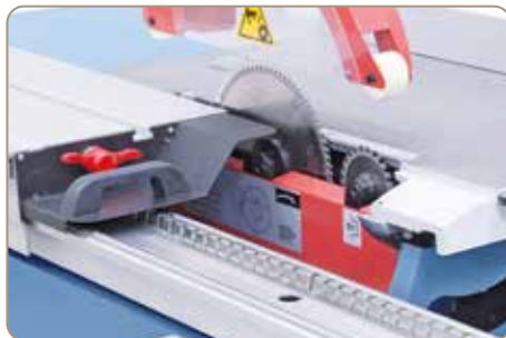
Complete with scoring unit for burr-free processing of sheet materials.
