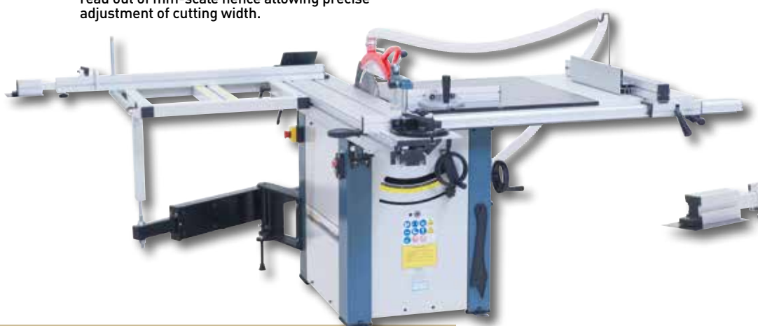
The magnifying glass on the rip fence ensures an easy read out of mm-scale hence allowing precise adjustment of cutting width.
