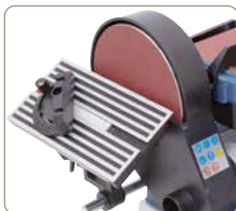
Sanding table tilts from 0° to 45°.
