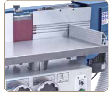
Grooved infeed ruler for excess veneer parts.
