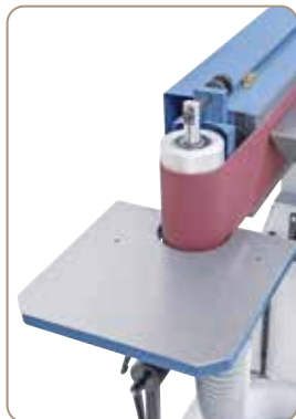
Rotary sanding table features dust port for ideal sanding of radius or contour.
