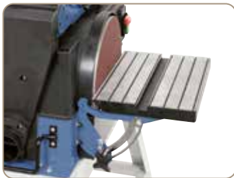
Aluminium support table can be tilted steplessly from 0° – 45°.
