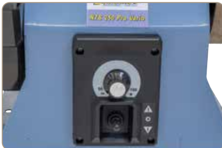
Supplied as standard with stepless speed control, ideal for adapting to the respective material
