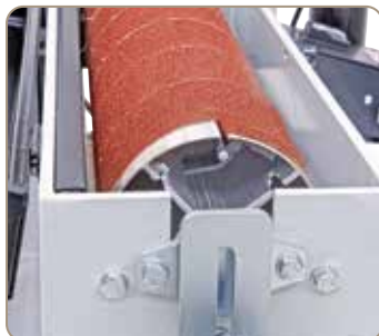
Quick clamp system for sanding belt.
