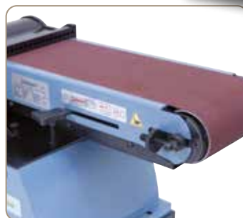
Large face sanding area with workpiece fence.
