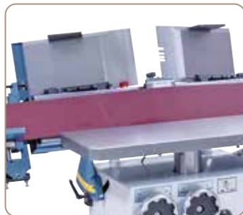
Quick folding up of sanding fences for sanding solid timber.
