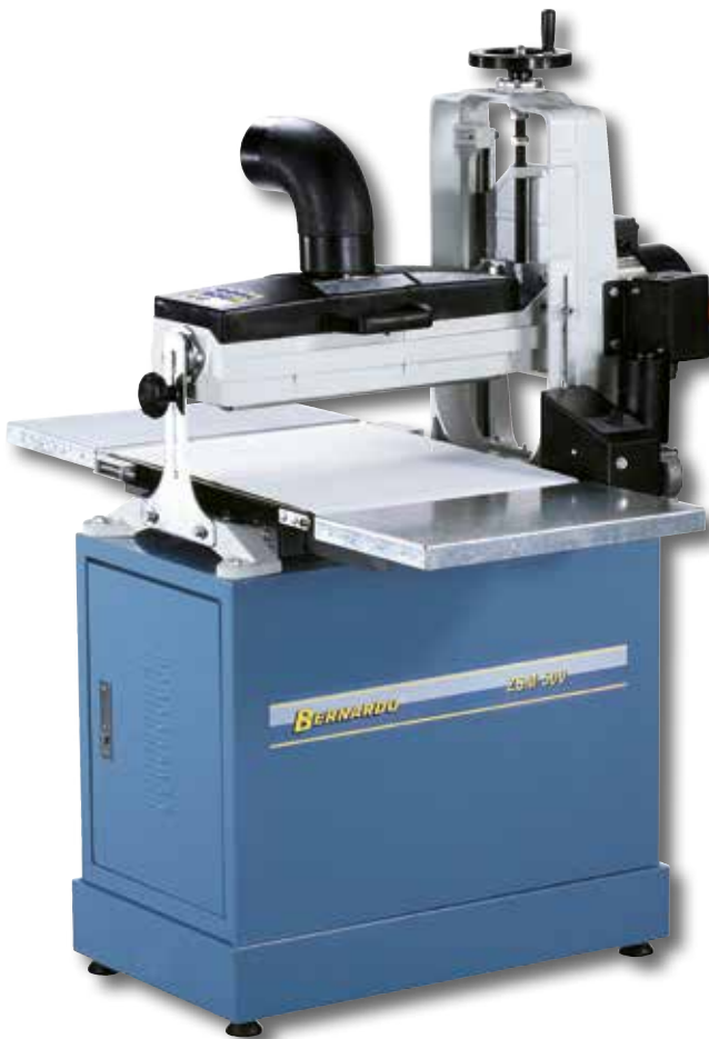
Quick clamp system for sanding belt.
