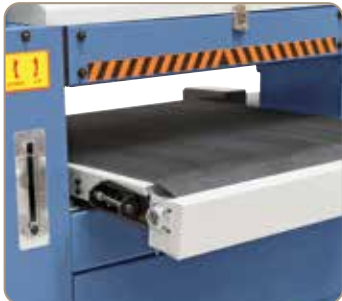
Adjustment screw for parallel run of the conveyor belt.
