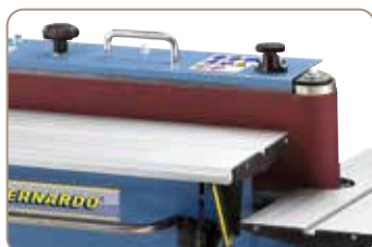
Height adjustable work table (up to 110 mm) ensures ideal use of sanding belt width.
