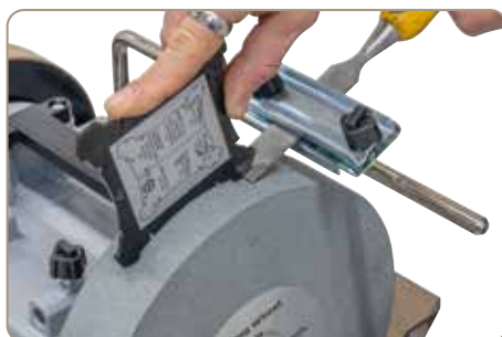
Easy angle adjustments by using the angle gauge WL-60 (standard).
