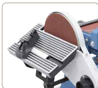
Sanding table tilts from 0° to 45°.
