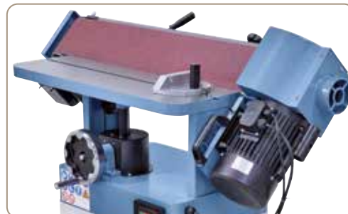
Sanding unit can be tilted steplessly from vertical to horizontal position.
