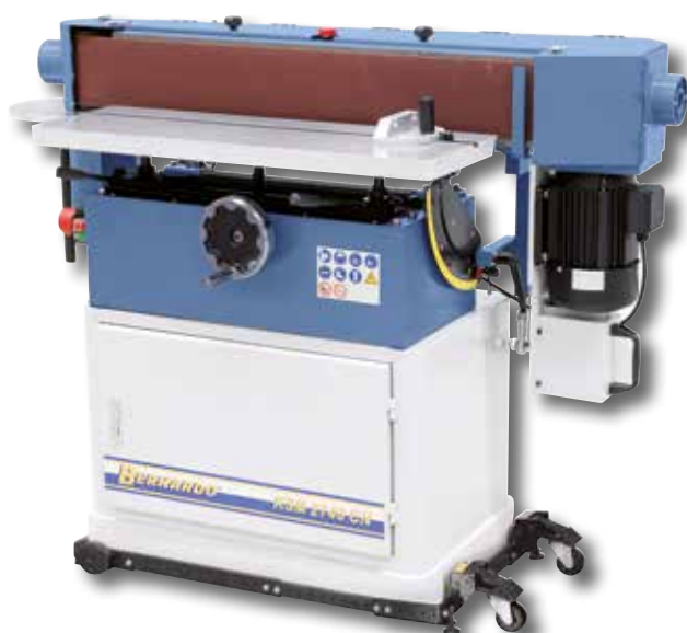
Universal mobile base allows for easy change of location. (optional extra)
