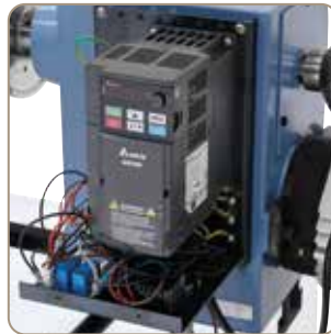
High-quality frequency converter allows for stepless adjustment of the spindle speed.
