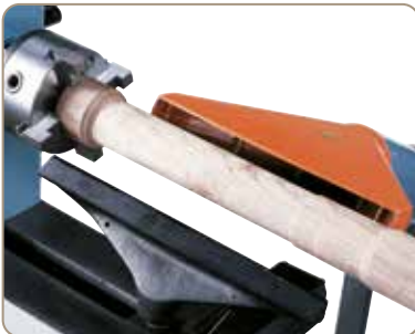
The optionally available dust extractor allows for clean working conditions.
