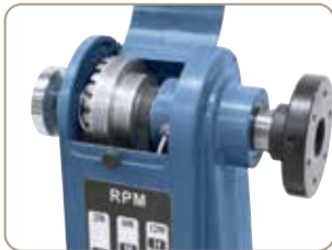
Repositioning the V-belt allows for easy change of the transmission ratio.
